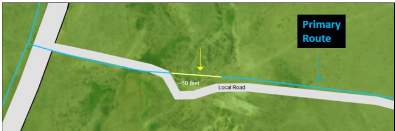
Figure 6. Example of a trenchless segment satisfying the Part 2 co-location criteria (e.g. avoiding a rock outcrop, short efficiency segment of 50 feet that rejoins the primary route, or even data error).
