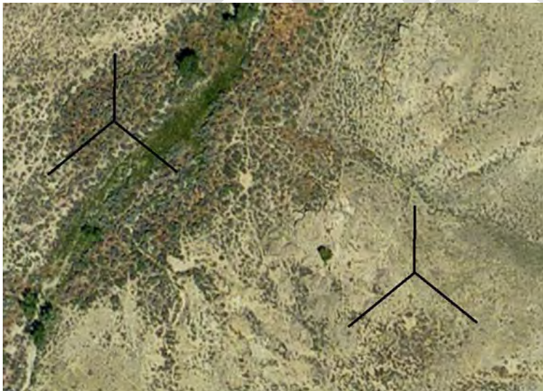
Figure 4. 4. Spoke Design will be used for non-linear projects (Herrick et al. 2016). Example of a project with an area larger than 20.0-acres, requiring two spoke design points with three 50.0-m transects each. Transects are located in a way to capture variation of dominant vegetation.
