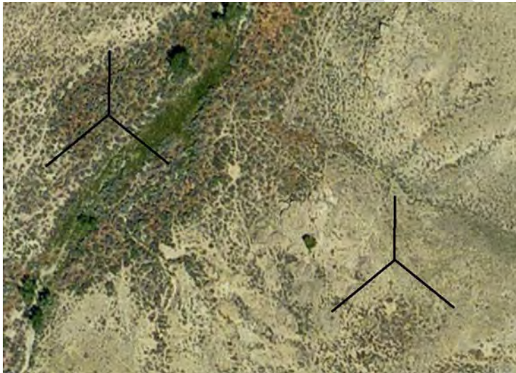
Figure 5. 4. Spoke Design will be used for non-linear projects (Herrick et al. 2016). Example of a project with an area larger than 20-acres, requiring two spoke design points with three 50-m transects each. Transects are located in a way to capture variation of dominant vegetation.
