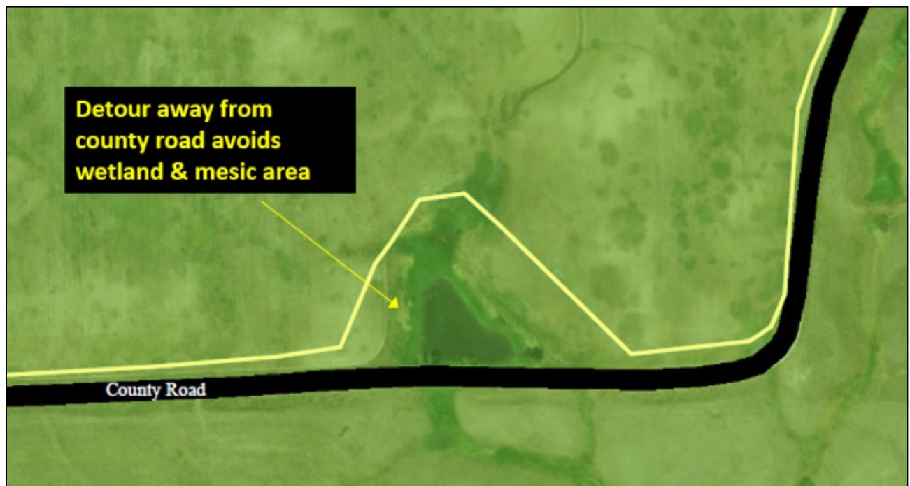
Figure 7. Example of a trenchless segment satisfying the Part 2 co-location criteria (e.g. detouring around a wetland and mesic area upstream) and re-joins the primary route.
